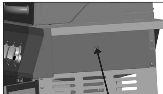
Hole for viewing the flame
