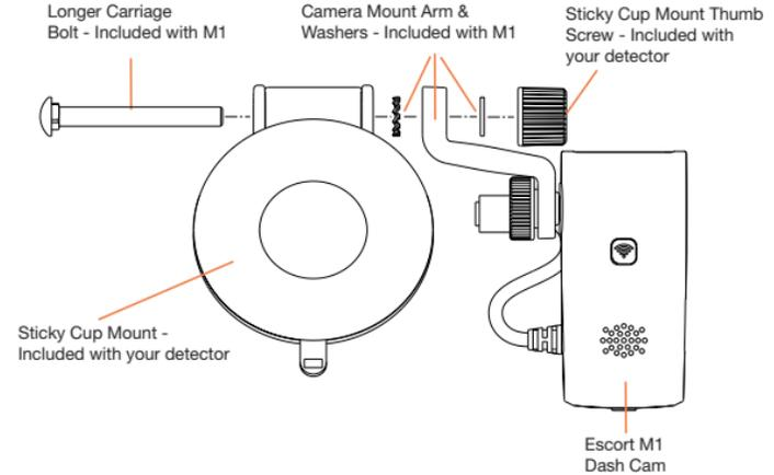
**Note:** Some components from your compatible detector's mount will be used. Your M1 is pre-mounted on the Camera Mount Arm.
