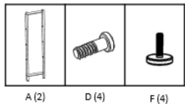
Screw ADJUSTABLE SHELF RESTS (D) into desired frame level (there are 3 levels for you to choose), make sure all 4 ADJUSTABLE SHELF RESTS (D) are on the same level.
