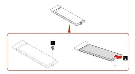
Note: The thermal pad is installed beneath the M.2 solid-state drive. Remove it if necessary.
