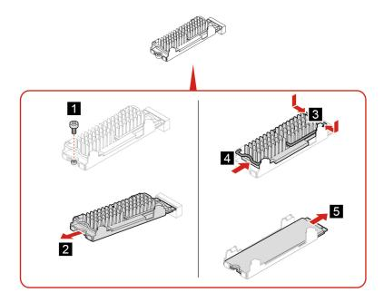
Note: Remove the film that covers the thermal pad (if any) when installing the M.2 solid-state drive, heat sink, and thermal pad.
