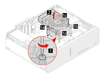
Note: To avoid the heat sink misalignment and the damage to the screw threads, the four screws on the heat sink should be fastened in sequence. First, fasten the top right screw half. Then, fasten the bottom left, bottom right and top left screw in sequence. Finally, fasten the top right screw well.
