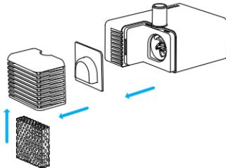
2. Remove the impeller by hand.
