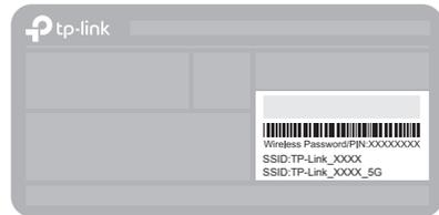
The default wireless network names (SSIDs) and password are printed on the label at the bottom of the router.
