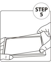
At an angle, place the edge of glass up against the inside of the guide frame and slowly lay the glass down onto the screen from left to right.
