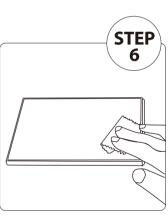
Remove the guide frame and push any air bubbles that may exist to the edge of the glass using the plastic card.
