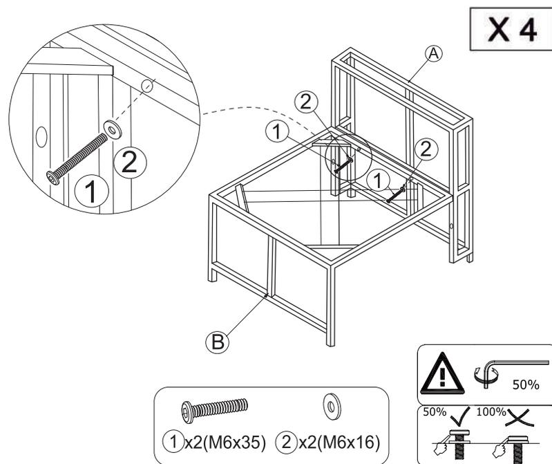
**EN:** Please don't fasten the screw completely during assembly process. It will be likely to lead to an assembling problem the screw hole position is not aligned. You can fasten completely when all parts have been assembled.
