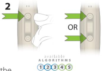
What you are doing is sampling the available acoustic settings for quiet environments. There are five different settings for you to try. Choose the one that sounds best to you – most natural, most helpful volume level. Press and release the upper or lower rocker switch to continue sampling the settings.
