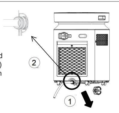
Note: The external drainage hose should not be too long (the recommended length is less than 0.6 m/2 ft). The height of the hose end must be at least 10 cm/4" lower than the drainage outlet on the machine. Ensure that the hose remains unobstructed, as it may otherwise result in improper drainage. Refer to the diagram below for clarification.
