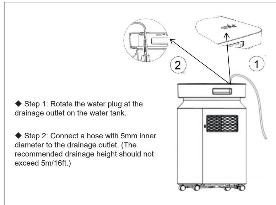
◆ Step 1: Rotate the water plug at the drainage outlet on the water tank.
