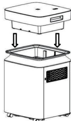
Note: When the water tank is full, please empty the water. Before putting the water tank back, please confirm that the float is working, and then use both hands to put the water tank in place.
