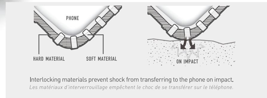
Interlocking materials prevent shock from transferring to the phone on impact.
