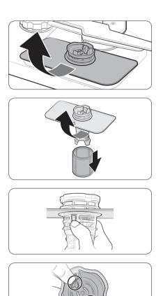
**3.** Remove the Coarse filter, and then the cylindrical micro filter underneath.
