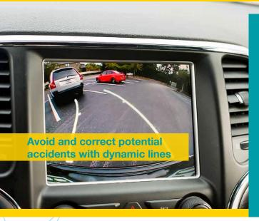
Relax in reverse. CAM-DPL features dynamic parking lines that move when you move. Simplifying maneuvering in even the most complex situations, the parking lines give you a clear understanding of the trajectory of your car before you reverse. The camera features built-in motion sensors, once the vehicle starts moving the camera senses the movement and the guidelines move to show the path of the vehicle.
