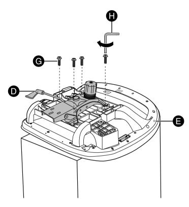
**6** With the seat still supported, align the holes in the bottom of the chair back with the bracket on the riser mechanism. Make sure that the arms are toward the front of the chair seat.
