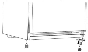
7 Install the leveling foot you removed from the left side into the right bottom of your refrigerator. 8 Install the bottom hinge and the door stopper on the right bottom of your refrigerator using the screws your previously removed. Tighten the screws.
