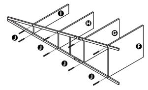
Attach the shelves to the *right* A-Frame by aligning the Shelves **OOOO** with the appropriate set of holes in the A-Frame and inserting 2 Screws **O** through the frame and into each Shelf as shown. Tighten using the Hex Key **O**.
