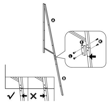
Finish assembling the first A-Frame by connecting the Back Frame Leg
