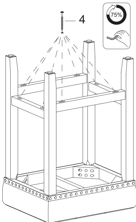
Secure the foot rests with the screws (Part 4).
