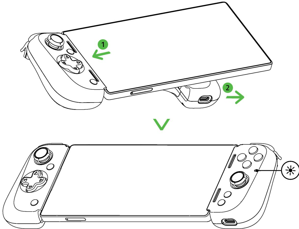
**i** Maximum supported dimensions: 11.5 mm (thickness, including camera) x 170 mm (Length)
