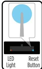
If the interface fails to function, press and release the reset button, then repeat the programming process from step 4 to try again.
