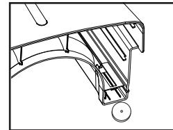
After the tank is emptied and placed back into position, the full tank protection will be released, and the indicator will turn off.
