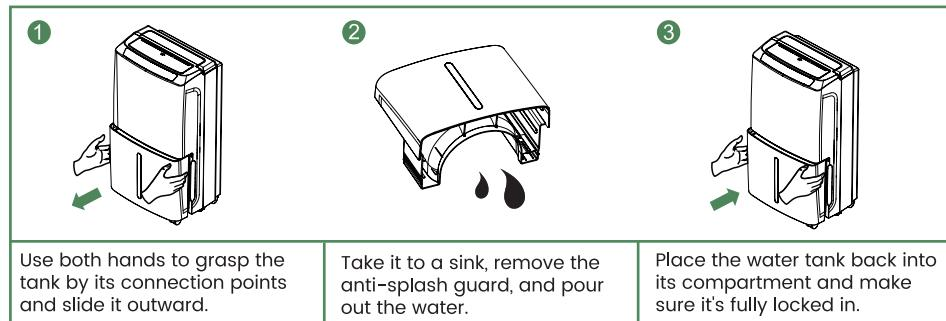
Use both hands to grasp the tank by its connection points and slide it outward.
