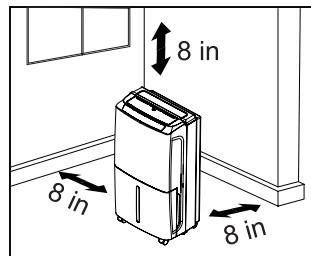
When positioning the dehumidifier, please ensure it is not placed too close to walls or other objects, as this could obstruct the air vents. Maintain a minimum clearance of 8 inches above and around the device, as depicted in the diagram.
