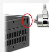
This is a small, metal-reinforced hole which is part of an anti-theft system. PN-SPCi7W10S provides an appropriate hole on both sides of its chassis.
