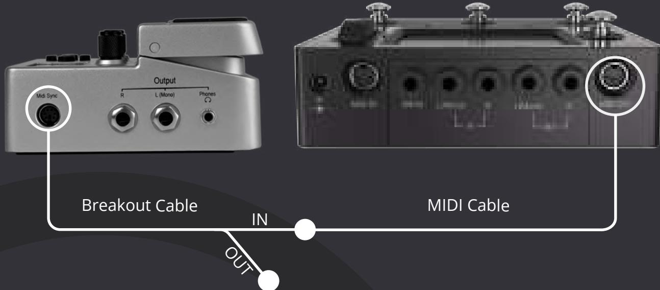
In both 2x2 and 6x6, starting the Aeros will start the BeatBuddy with an intro fill or with the main beat, if the intro fill has been disabled on the BeatBuddy (to disable the intro fill go to Main Pedal > Intro > None), and stopping the Aeros will stop trigger an outro (unless the outro is disabled), stopping the BeatBuddy and Aeros at the end of the measure.
