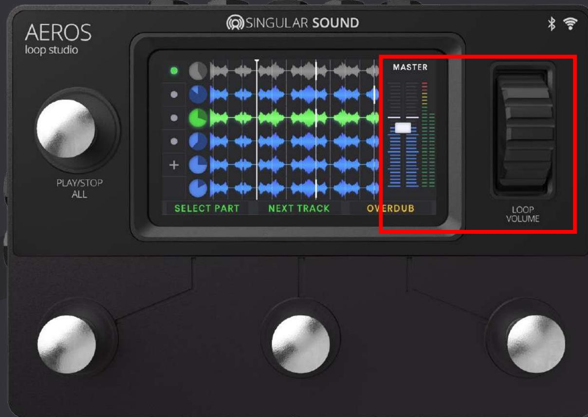
The thin bars on the right show the L and R input volume levels. If the bars are red you are clipping and should lower the volume of your instrument.
