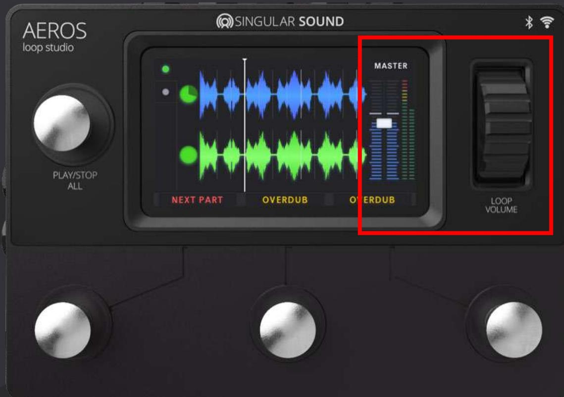
The thin bars on the right show the L and R input volume levels. If the bars are red you are clipping and you should lower the volume of your instrument.
