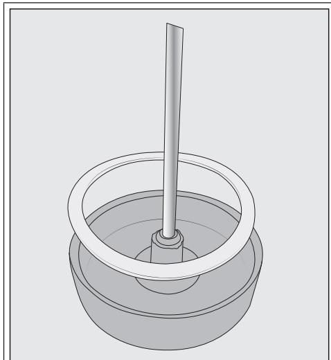
If necessary, you can remove the connecting piece and seal from the milk flask lid. Once you have removed the stainless steel tube, the connecting piece is easy to push out from the inside of the lid.
