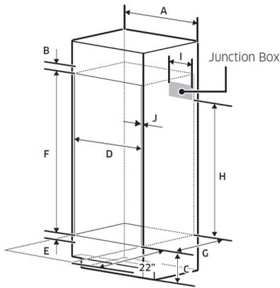
Allow a minimum of 22" for clearance to adjacent corners, drawers, walls, etc. when door is open
