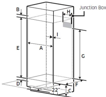
Allow a minimum of 22" for clearance to adjacent corners, drawers, walls, etc. when door is open.
