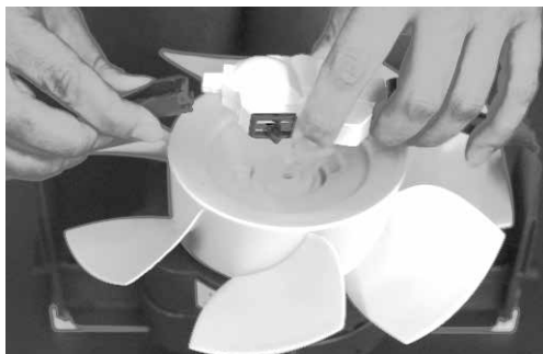
Fig 6. ... gently pull one of the motor assembly arm 1/8 inch ...
