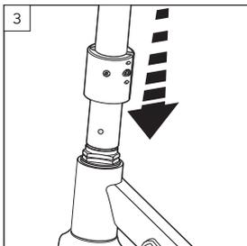
Slide down collar down until it bottoms out on the main frame.
