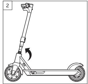
Align oval tube and fork stem shaft bolt holes. Align holes by rotating the oval tube until it is aligned with the fork stem.
