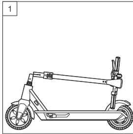
Rotate oval tube and align opening with the fork stem shaft.
