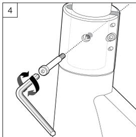
Ensure collar hole aligns with fork stem and oval tube holes. Once aligned, insert the M5 shoulder bolt and tighten. Tighten until shoulder bolt no longer rotates.
