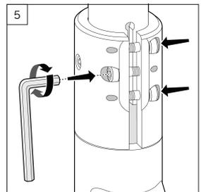
Tighten all 3 collar screws. To avoid serious injury, the three collar screws must be tightened securely before riding.
