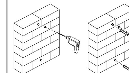
**CAUTION:** To prevent property damage or personal injury, never drill into the mortar between blocks. Mount the wall plate directly onto the concrete surface. Align the center of the template at the height determined in Step 4 of the User Guide. Make sure that it is level, then tape it to the wall.
