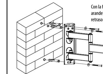
With the arrow on the wall plate pointing up, align the plate with the anchors, then insert the lag bolts through the washers and wall plate holes and into the anchors. Make sure that the wall plate is level, then tighten the lag bolts.
