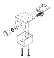
Disassemble the ACR-3 from its mounting bracket. Drill a 9/32" (7 mm) hole in the dashboard for the control along with a 3/32" (2.3 mm) hole for the lock tab and 1/8" (3 mm) holes for the LEDs. Make sure that you do not drill though any wires or other components. Reassemble the dash control components on the dashboard.
