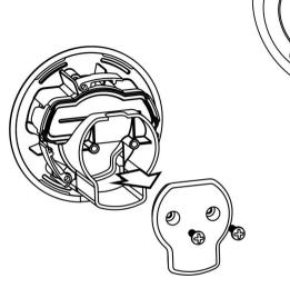
Insert the power harness plug into the back of the bottom module and re-secure the back cover.
