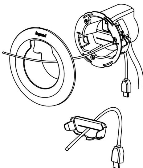
**NOTE:** The gasket can be removed if desired to allow for cables with larger connectors to fit through the opening.
