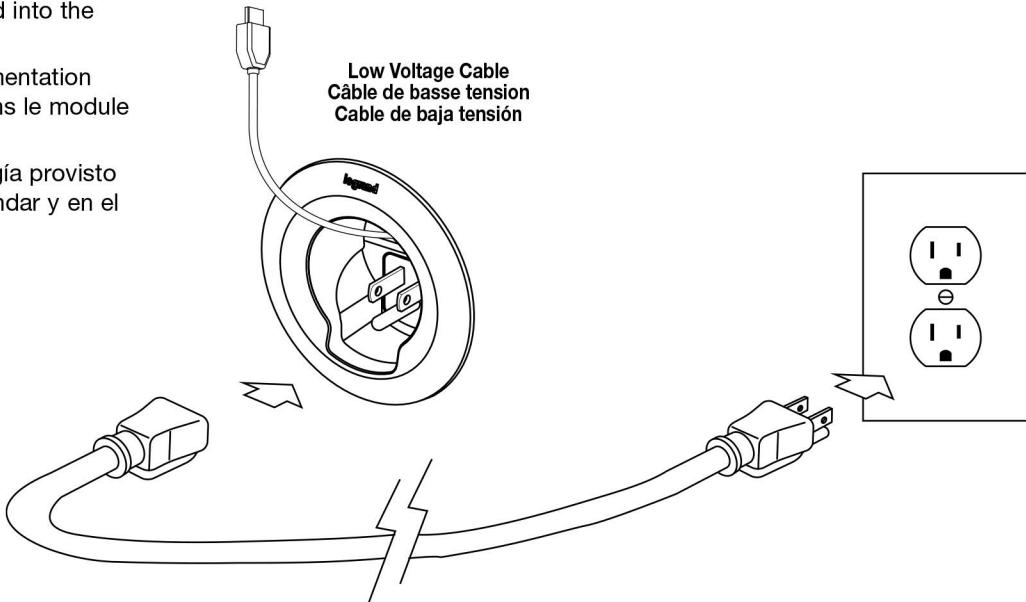
**CAUTION:** Risk of fire. Do not install power supply cord within the wall cavity.
