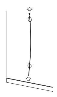
Hook the wire of the Power Harness to the fish hook and pull through the wall until it protrudes through the bottom hole.
