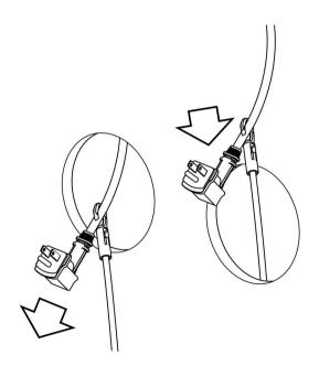
Unsnap the trim ring from the pre-assembled upper module. Route low voltage cables through the upper module and gasket. Route the low voltage cables through the upper hole and out through the bottom hole. The fish tape may also be used to help route the cables.
