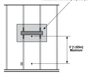
Measure and mark the center of each hole location. The top and bottom assemblies can be located a maximum of 5 feet apart within the same wall cavity.
