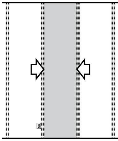
**NOTE:** Exterior walls with blown-in type insulation may require removal of some of the insulation within the wall cavity.
