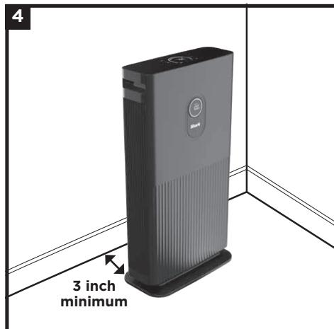
Set up the unit on a level floor surface, at least 3 inches away from walls. Plug unit in and power on.
