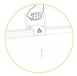
5. When finished, lift up on the handle to release the screen and slowly lower it into the case.
