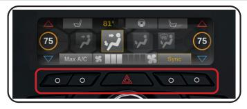
**If popups are turned on in the menu:** The proximity sensor, within the dash bezel, will display the descriptive tabs when your hand is near the buttons. When your hand is removed, the tabs will disappear.
