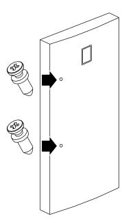
**3** Loosen the hex screws on the top and bottom of the handle with the hex wrench (provided) so that you can fit the handle over the extended head screws in the door.
