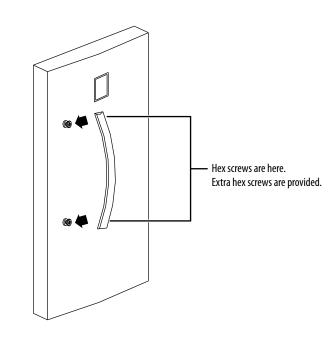
**4** Place the door handle over the heads of the screws, then tighten the hex screws.
