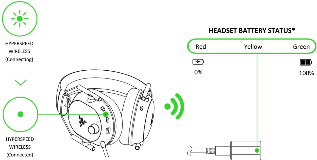
*\*By default, the dongle indicator LED will display the headset's battery status when connected via Razer HyperSpeed Wireless (2.4 GHz) mode. You can customize the indicator LED to show the headset's connection status, battery status (default) or low battery warning only from the Razer Synapse app. [Learn how to customize the dongle indicator LED](#)*
