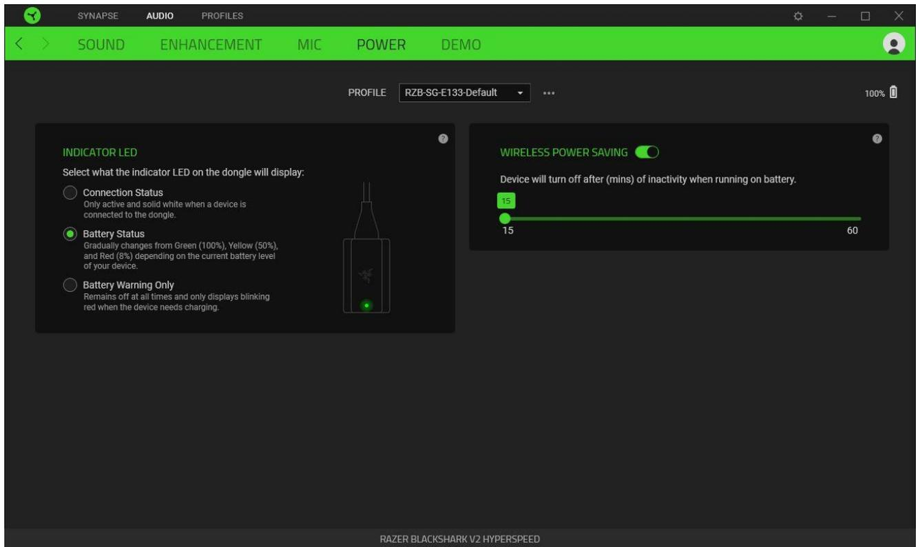
**!** *By default, the indicator LED on the wireless dongle displays the headset's battery status.*
