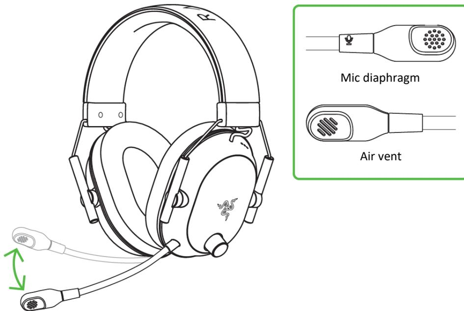
**i** The recommended mic-to-mouth distance for optimal sound capture is 1.5 cm to 3 cm (0.59 in to 1.18 in).
