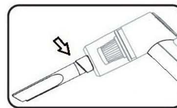
**Brush Tool:** For use on surfaces requiring softer surface cleaning. Can connect to crevice tool as shown in diagram or to main body directly.
