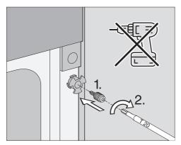
Insert the bolt into the mounting aid and tighten it in the cabinet niche. Do not use a cordless screwdriver.
