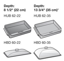
\* The casserole dish cannot be used in conjunction with this lid in ovens with 3 shelf levels because the total height would exceed the height of the oven cavity.
