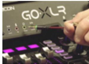
**Pro Tip:** You may also run your headphone cable underneath GO XLR by using the cable channel designed into the underside of the unit, so that you do not have to wrap your headphone cable around the GO XLR mixer.
