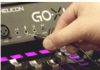
4. If your microphone does not have an XLR connection, you can connect the microphone to the MIC input with the pink ring immediately to the right of the LINE IN jack. This MIC connection can also work with the Blue Yeti\* microphone.
