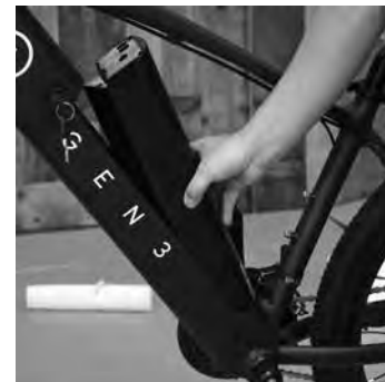
Align battery with the receptacle and snap into place
