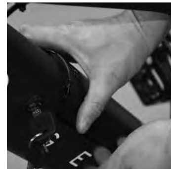
Unlock battery with key and remove battery for charging
