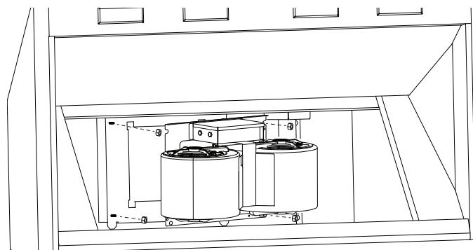
2. Attach (4) nuts (included with hood) to the weld studs. Tighten nuts to secure the blower to the hood.
