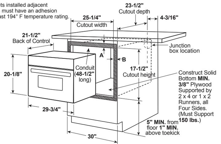
A= Allow 1" overlap of oven over bottom edge of cutout, and allow 2-3/4" overlap at top edge of cutout.
