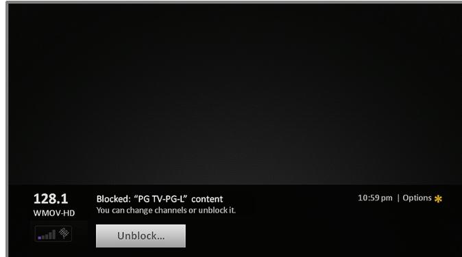
Whenever this blocked message appears, both the video and audio of the show are blocked, as well as program data that would normally appear in the area at the bottom of the screen.
