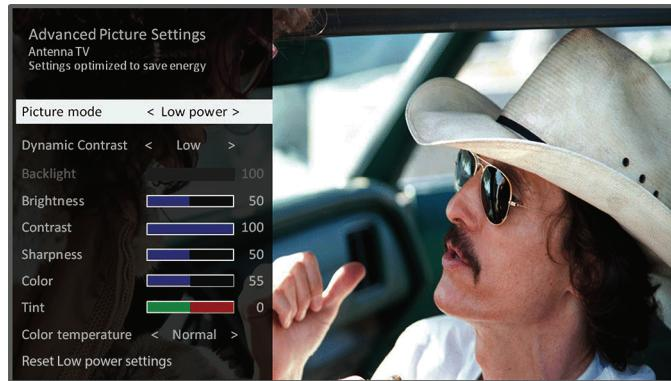
To adjust the settings on the **Advanced Picture Settings** menu, press the **UP** or **DOWN** arrow to highlight a setting, and then press the **LEFT** or **RIGHT** arrow to change the setting. You'll notice the changes you make right away in picture appearance.
