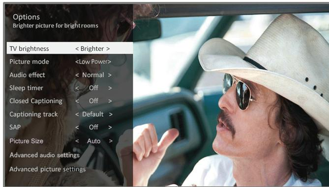
To adjust the settings on the *Options* menu, press the **UP** or **DOWN** arrow to highlight a setting, and then press the **LEFT** or **RIGHT** arrow to change the setting. You'll notice the changes you make right away in picture appearance or audio quality.
