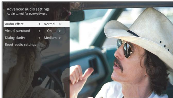
To adjust the settings on the *Advanced Audio Settings* menu, press the **UP** or **DOWN** arrow to highlight a setting, and then press the **LEFT** or **RIGHT** arrow to change the setting. You'll notice the changes you make right away in sound quality.
