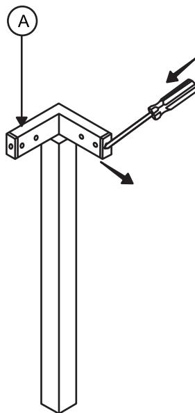
**EN:** Insert a screwdriver into the plastic plug hole and pry out.
