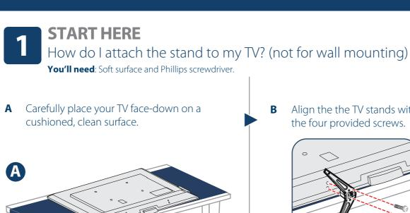
Align the TV stands with the screw holes on the bottom of the TV, then secure the stands to the TV with the four provided screws.  $M6 \times 36 \text{ mm screws}$ Right Left
