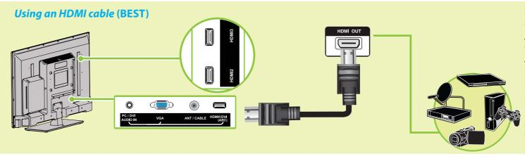
Multipurpose jacks: You can plug any device that uses HDMI into any HDMI jack. However, certain devices must be connected to the HDMI1/DVI (ARC) jack. See the instructions that came with your ARC or DVI device for more
