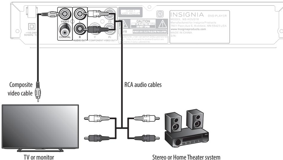
**3 Composite or Component:** Plug the white (left) and red (right) connectors from an RCA audio cable to the **L** and **R AUDIO OUT** jacks on your DVD player to the white (left) and red (right) audio in connectors on your TV, monitor, stereo, or home theater system.
