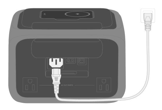
It's recommended that you use a power socket with a capacity of more than 10A and ensure that the working current of the socket is constantly greater than 10A.
