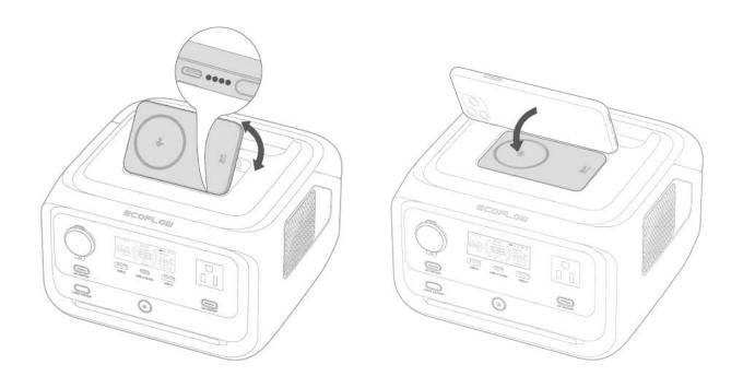
When attaching the power bank, ensure the pogo pin ports on both devices are properly aligned and connected.
