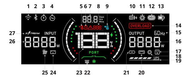
**On**: The power station is connected to the internet via Wi-Fi.
