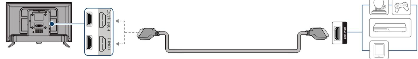
**Multi-purpose jacks:** You can plug any device that uses HDMI into any HDMI jack. However, certain devices must be connected to the **HDMI 1 (ARC)** jack. See the instructions that came with your ARC device for more information.
