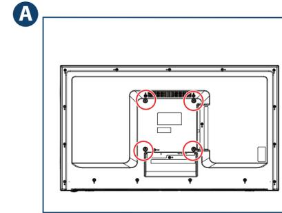
**B** Your TV has four VESA mounting holes on the back. If you attach a wall-mount bracket to the back of your TV, **the bracket must be securely attached, using all four holes.** If you do not use all four mounting holes, your TV may fall and cause property damage or personal injury. See the documentation that came with your wall-mount for complete mounting instructions.
