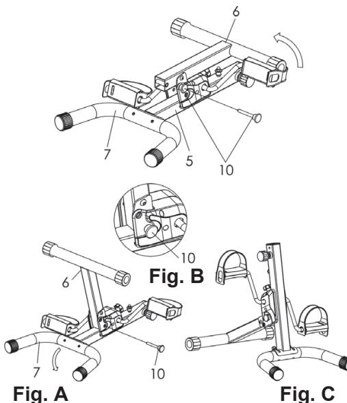
**EN:** Pull the bolt (No. 10) out of the main frame (No. 5) and then turn the rear pin (No. 6) according to the arrow direction into the position in Figure A. Insert the bolt (No. 10) into the main frame (No. 5). The position for inserting the bolt (No. 10) is shown in Figure B. Finally, connect and secure the front fork (No. 7) and main frame (No. 5). The structure shall correspond to the information given in Figure C.
