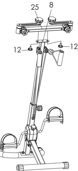
**EN:** Using rotary knob (No. 12) to secure crankshaft (No. 25) on main frame (No. 5) and tighten it securely.
